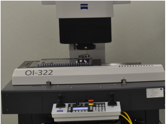
Zeiss CMM that inspects with probes and optics
